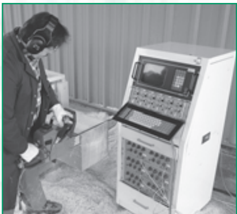
Accelerometers placed on each handle convert vibrations generated during test cuts into electrical signals. The signals are fed into specialized computer systems for analysis.
