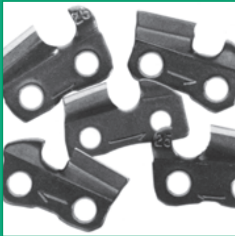
Oregon® Vibe-Ban™ low-vibration chains are easy to identify; they're stamped with a forward-pointing spear on the outsides of cutters.
