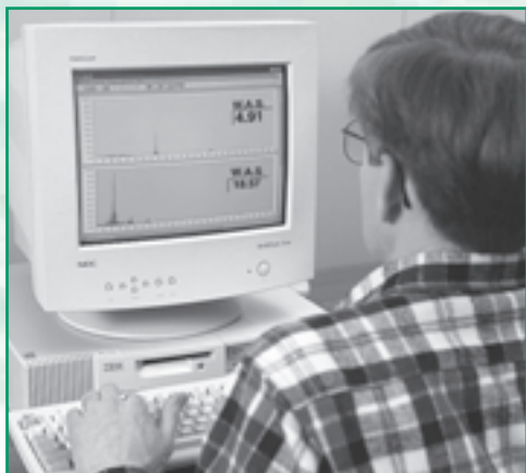
These two graphs give a pictorial comparison of two saws' test results. The ultimate measurement "W.A.S." stands for "Weighted Acceleration Sum." The lower the W.A.S., the better.
